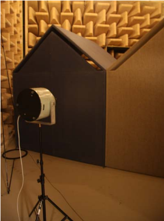
Picture 1 – Test arrangement for measurement of The Hut – at joint. The loudspeaker is shown in the picture.
