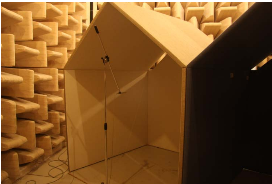
Picture 3 – Test arrangement for measurement of The Hut – inside the house. The standard microphone position is shown in the picture.
