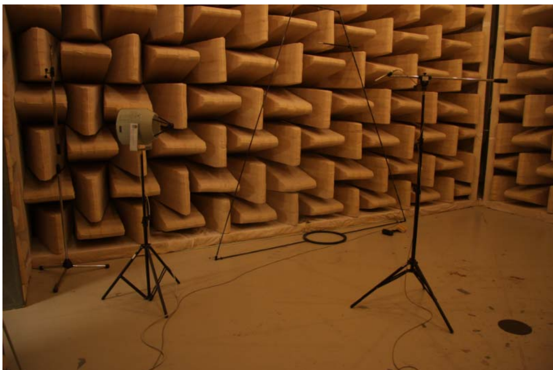
Picture 4 – Test arrangement for measurement of reference microphone position for The Hut – at joint.
