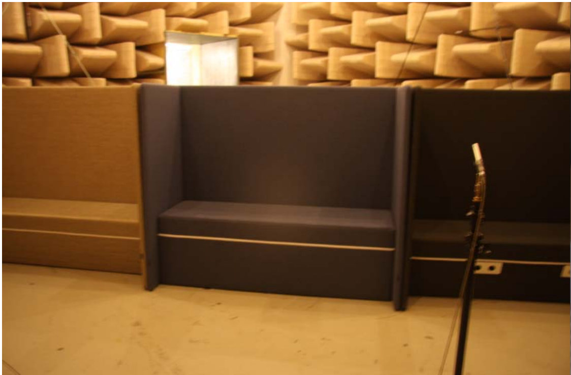
Picture 6 – Test arrangement for measurement of Sofa Sound Booth. The standard microphone position is shown in the picture.
