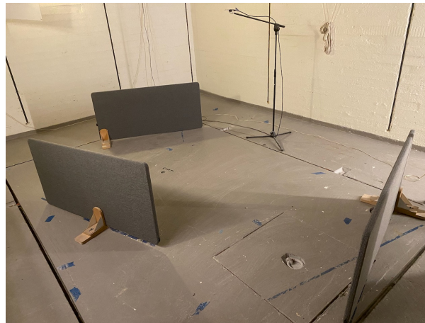
Figure 2: Three ScreenIT A30 Core 1400 x 650 mm measured for sound absorption area.
