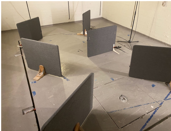
Figure 1: Six ScreenIT A30 Core 800 x 650 mm measured for sound absorption area.
